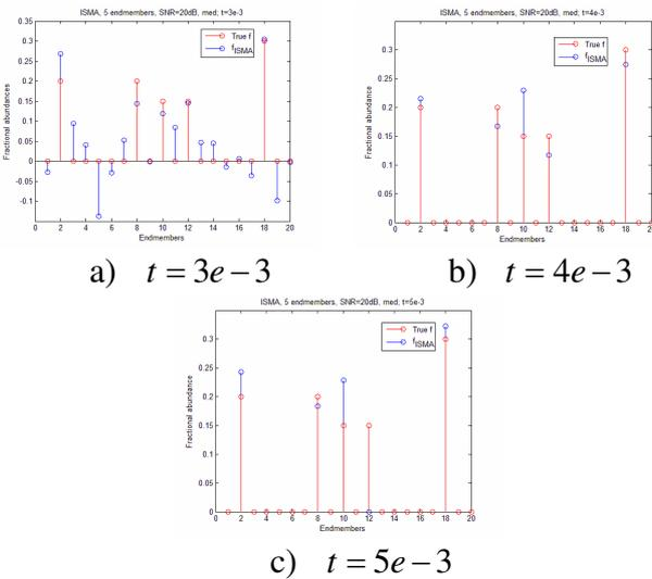
Fig. 2 ISMA - the reconstructed fractional abundances for different thresholds  $t$ .
