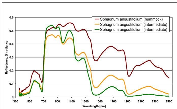
Fig. 2. Reflectance spectra of *S. angustifolium* in different moisture level
