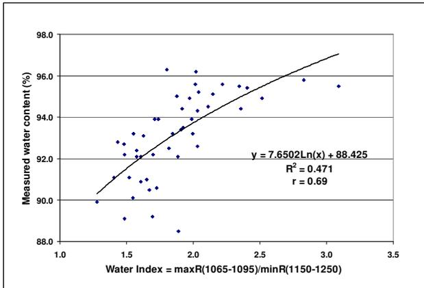
Fig 5. Logarithmic correlation between measured water content and calculated WBI of *Sphagnum* species.
