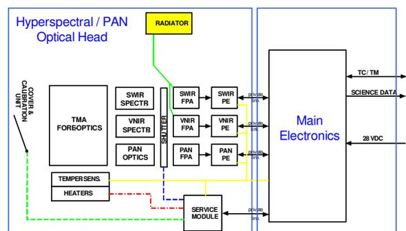
Fig. 4 – PRISMA Instrument block diagram
