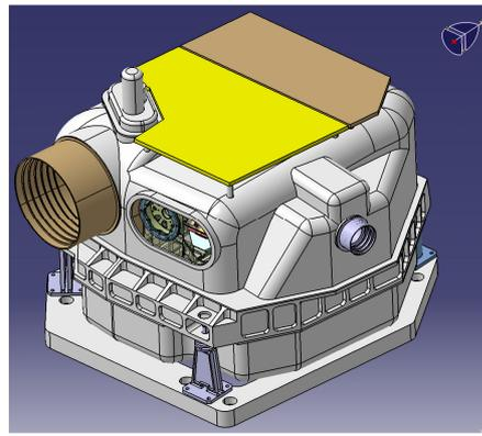
Fig. 5 – Hyperspectral / PAN Optical Head layout
