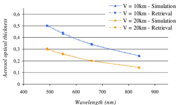
Figure 7. Comparison of the AOT used to perform the Amartis v2 simulations and of the mean results of the retrievals, for the two visibilities.
