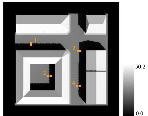
Figure 6. Simulated at sensor radiance image (in  $W.m^{-2}.sr^{-1}.\mu m^{-1}$ ) at 660nm for a 20km visibility and the 4 “shadow/sun” pixels couples selected for the aerosols characterization.
