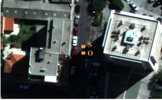
Figure 3. Example of sunny (S) and shadowed (O) pixels that can be used in the retrieval procedure.
