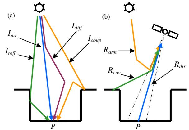
Figure 2. Components of the signal, at ground level (a) and at sensor level (b).
